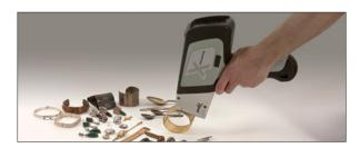
The DELTA can automatically identify and characterize a wide range of alloys, including precious metals such as Au, Ag, Pt, and Pd. It can be preprogrammed to provide on-the-spot gold karat classification, 0-24 kt.
