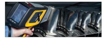
The DELTA can take results and compare them to a library of alloy compositions to "match" an unknown material to known alloys. Pop up messages can be preprogrammed for immediate sorting or coding instructions to increase efficiency and throughput.
