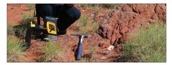
The DELTA metal and light element compositional results can be transferred wirelessly for XRF-GPS-GIS "instant geochemistry". It provides the ability to map, visualize, assess, and follow up on targets immediately for better mining exploration decision making.
