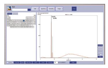
The energies (keV) at which the peaks appear identify the elements present in a material. The intensities (counts/s) of peaks correlate with the concentrations of the elements present in the material.
